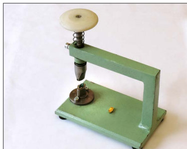
Device for prong closing when setting bigger stones
