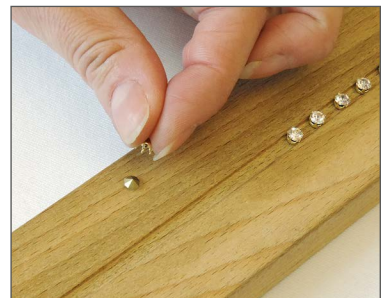
A simple tool with one groove for manual stone setting
