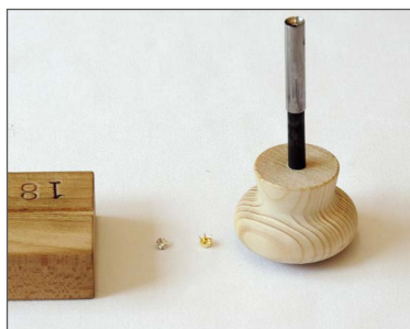
Setting and closing tool for individual cups
