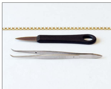
Tools for closing the cup by hand
