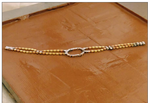
12 After soldering, let the product cool down.
