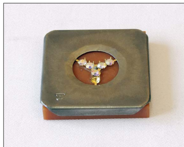
Device for manual setting of rhinestone balls
